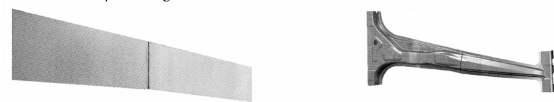
Figure 1. Tailored Blank for B-pillar
